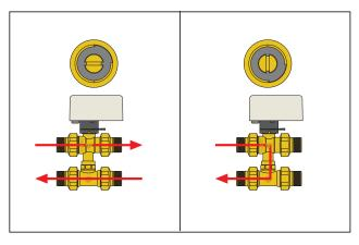
All the valves are supplied with the slot/indicator in the horizontal position.
