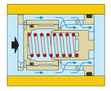
In this case, the regulating piston remains in equilibrium without compressing the spring and gives the medium the maximum free flow area. In practice, the piston acts as a fixed regulator and thus the flow through the AUTOFLOW depends solely on the differential pressure.
