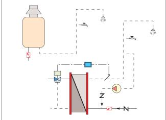
To limit the flow rate of hot water which can be delivered in systems with instantaneous production or limited capacity
