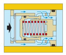
If the differential pressure is contained within the control range, the piston compresses the spring and gives the medium a free flow area to permit regular flow at the nominal rate for which the AUTOFLOW is set up.
