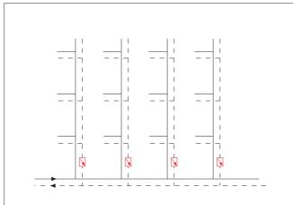
To regulate the flow rate in each riser or secondary branch of a system.
