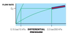
$Kv_{0.01} = 0,070 \cdot G_0$  Range  $\Delta p 15-200 \text{ kPa}$  where  $G_0 = nominal \text{ flow rate}$
